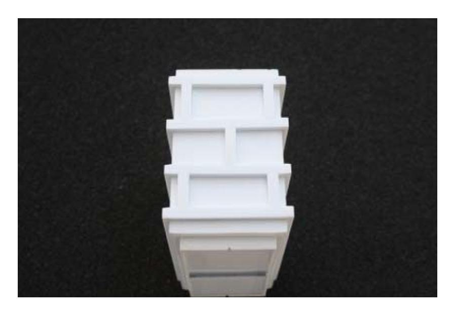
Finished "box" - Use putty on ribs to fill any problem areas and wet sand – be CAREFUL sanding around the control panel
